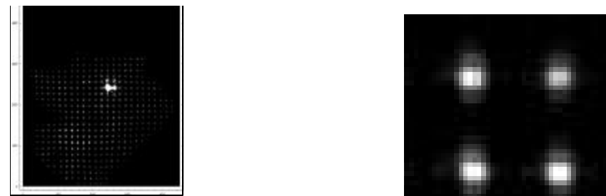
Figure 3.6: RK eye, high resolution. This image was from an RK patient with very bad lateral, non-symmetrical cuts. While the cuts did not protrude into the optical zone, the resulting wavefront is seriously aberrated. The pupil in this case was 4.8 mm, with effective 210 \mu\text{m} resolution lenslets. Note that the focal spots are still extremely well formed and precise, even for this highly aberrated input wavefront.
